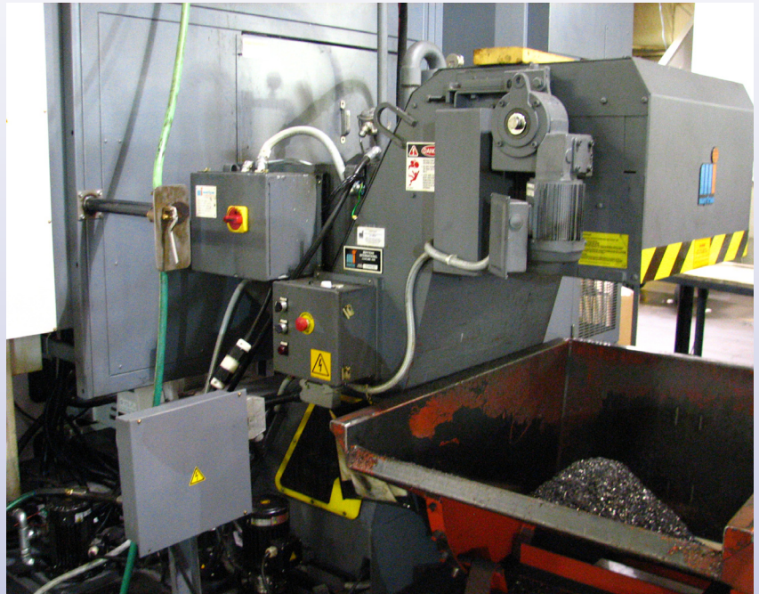
The Mayfran ConSep conveyor-separator has helped Team Industries reduce downtime while improving tool chip/coolant processing.
